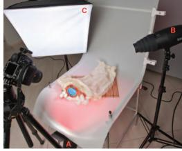
**Exposure data:**Nikon D800, Sigma 70mm Macro, 1/160s, f/11, ISO 100, power output: A-1/8, B-1/2, C-1/4
