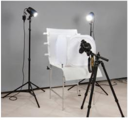
Both flashes are positioned so as to illuminate the back wall of the photo tent, which is reflected in the shiny metal surfaces.
